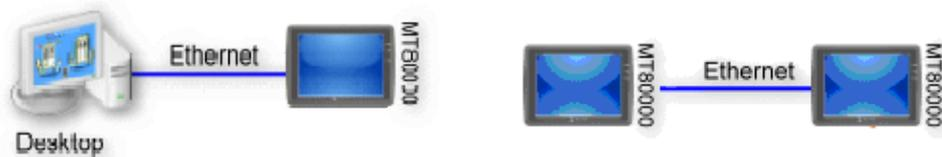
So-called “remote HMI” means through network, local HMI or on PC run on-line simulation to control remote HMI. To control a remote HMI should add this type of device. Click [New...] and the following [Device Properties] dialog display. Correctly fill in all of the properties as required.
