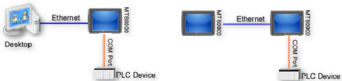
So-called “remote PLC” means a PLC is connect to a remote HMI. To control a remote PLC should add this type of device. Click [New...] and the following [Device Properties] dialog display. Correctly fill in all of the properties as required.
